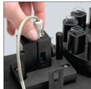
The temperature measurement kit provides precise in-cell temperature monitoring with real-time display within UV WinLab.
