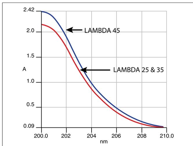
Figure 1. LAMBDA systems exceed the pharmacopeia stray light test specification of an absorbance of  $> 2.0A$  at 200 nm using a 1.2 w/v potassium chloride solution. The additional pre-monochromator in the LAMBDA 45 further reduces stray light compared to the LAMBDA 25 and 35.
