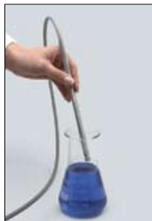
The fiber optic probe enables in-situ sampling away from the instrument.
