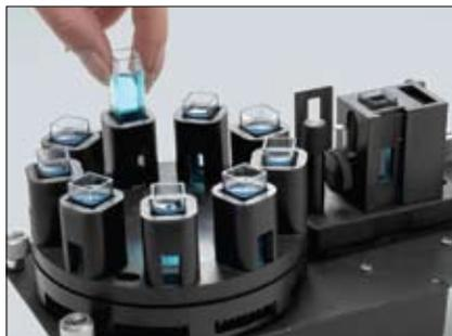
Peltier controllers accurately control the temperature of your experiment.
