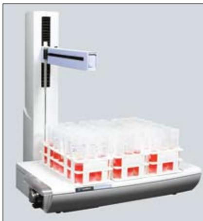
The S10 autosampler with built-in peristaltic pump offers unattended high-throughput measurement of up to 200 liquid samples. A wide range of sample vessels are available.
