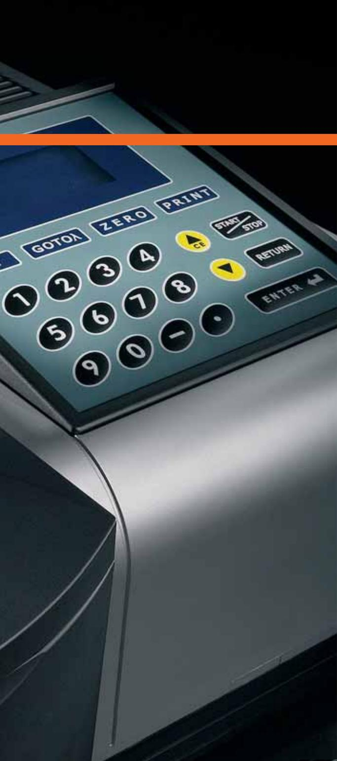
The T60 is a high performance compact split beam spectrophotometer with a fixed 2nm spectral bandwidth.
