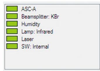
▶ The internal status monitor function offers continuous monitoring of the beam splitter type, the light source, the He-Ne laser, humidity condition, and information related to auto-start accessories.
