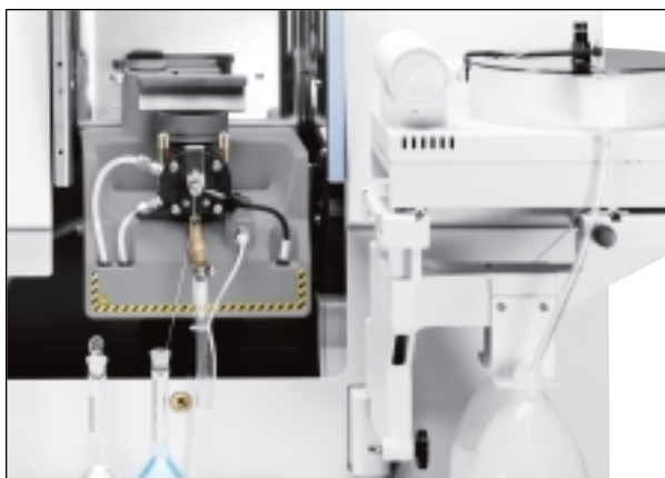
Figure 6. The AS-800 Furnace Autosampler easily swings out of the way for flame analyses.
